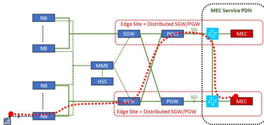
Figure 14: Example of tromboning with Distributed GWs
