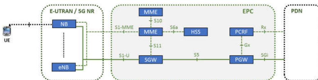
Figure 6: Non-roaming architecture for 3GPP access
