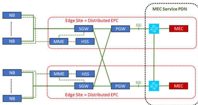
Figure 12: Example of two Distributed EPCs for one MEC Service
