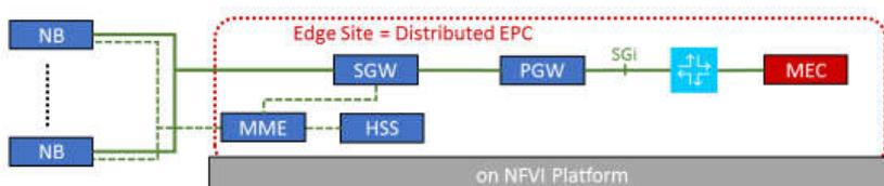
Figure 13: Example of EPC functions and MEC server on one NFV platform
