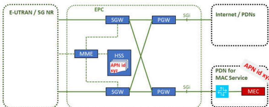
Figure 18: Example of a PDN being accessible via a (dedicated) PGW
