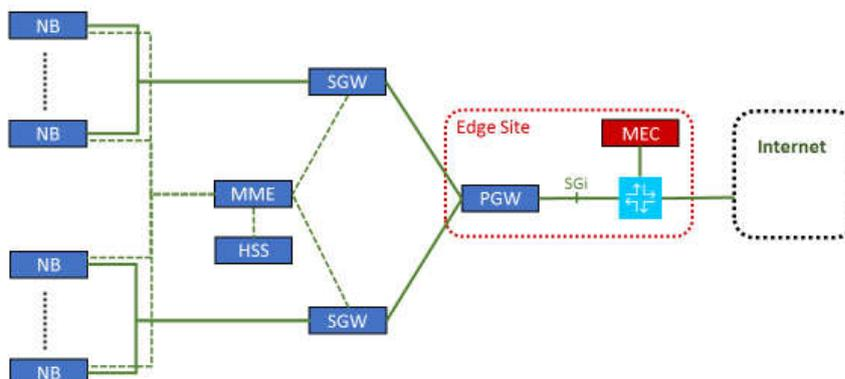
Figure 10: Example of an Edge Site at the edge of a cellular core network
