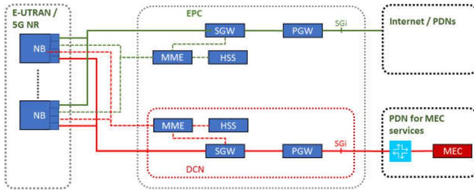
Figure 17: Example of a DCN within an EPC
