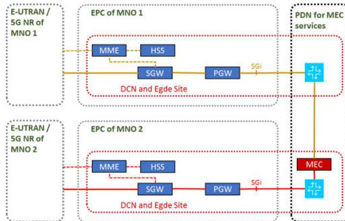
Figure 19: Example of Network Slicing (here DCN) and Edge Computing combined
