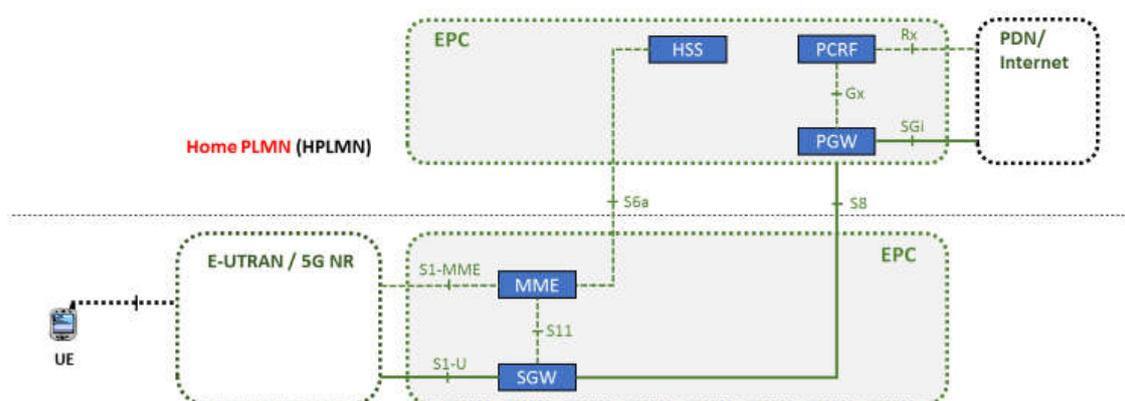
Figure 7: roaming architecture for 3GPP access: home routed traffic
